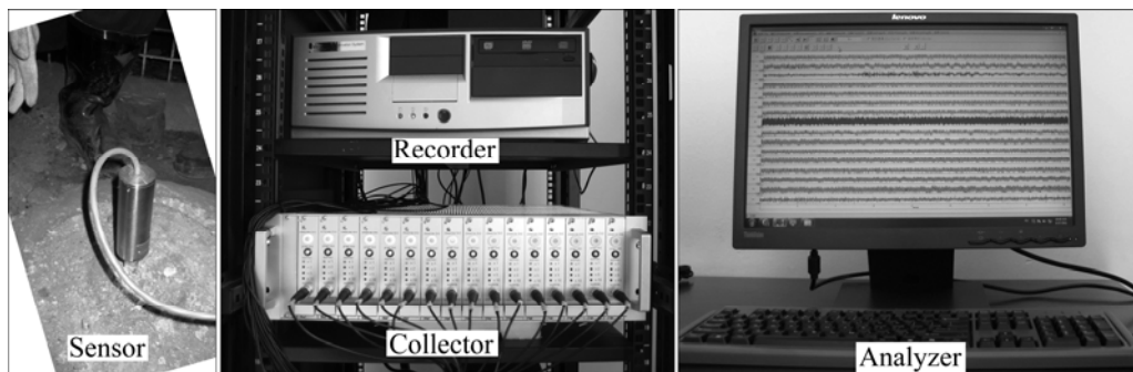
Fig. 7 Photos of SOS micro-seismic monitoring system
