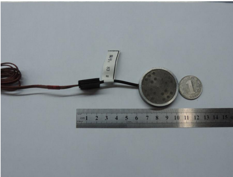
Solid pressure sensor
