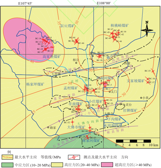
图7 宁正-彬长煤矿区最大水平主应力分布 Fig. 7 Distribution of the maximum horizontal principal stress in the Ningzheng-Binchang mining area
